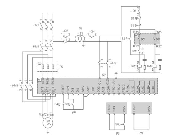
Connection in line, with line and bypass contactor, freewheel or controlled stop, type 1 or 2 coordination, non reversing, 2-wire or 3-wire
